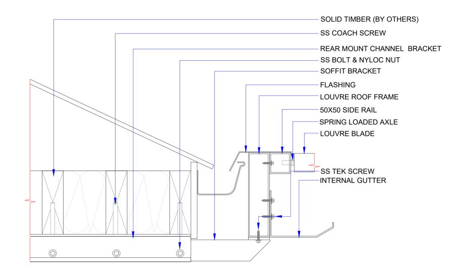
CROSS SECTION VIEW LOUVRE ROOF TO SOFFIT BRACKET FIXING DETAILS
