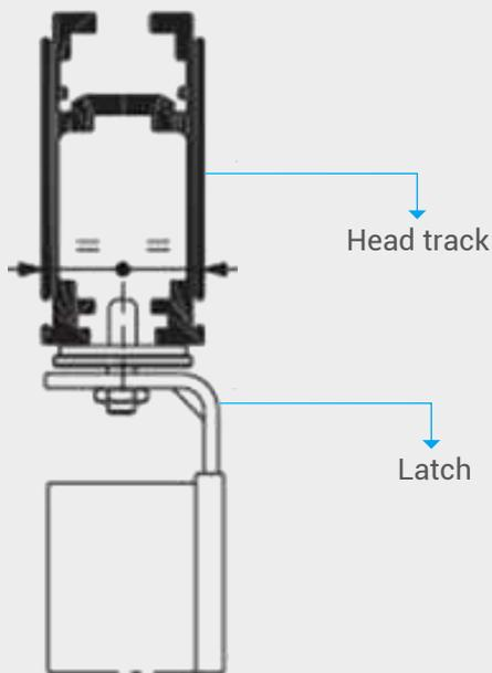
Shutter bolt for locking the screen in any position on the track. Specific head track details are required for this latch, contact the design team to discuss
